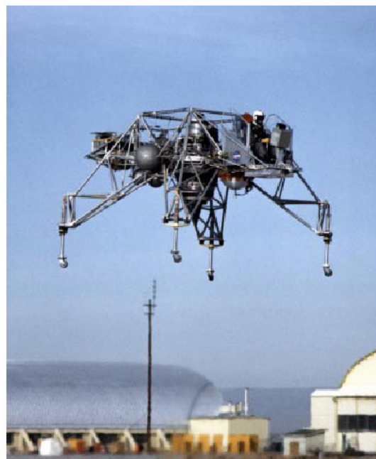
A Lunar Landing Research Vehicle is maneuvered during a test flight in 1964. NASA Photo ECN 506
